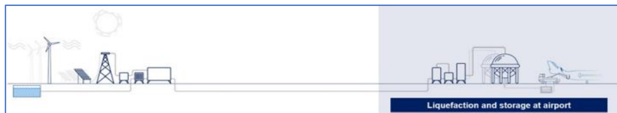
Figure 15: Scenario 3 — Hydrogen produced and liquefied locally at the airport (courtesy of ATI). Note: Renewable methods of onsite hydrogen production could be electrolysis, pyrolysis, etc., which require a grid and renewable power source.
